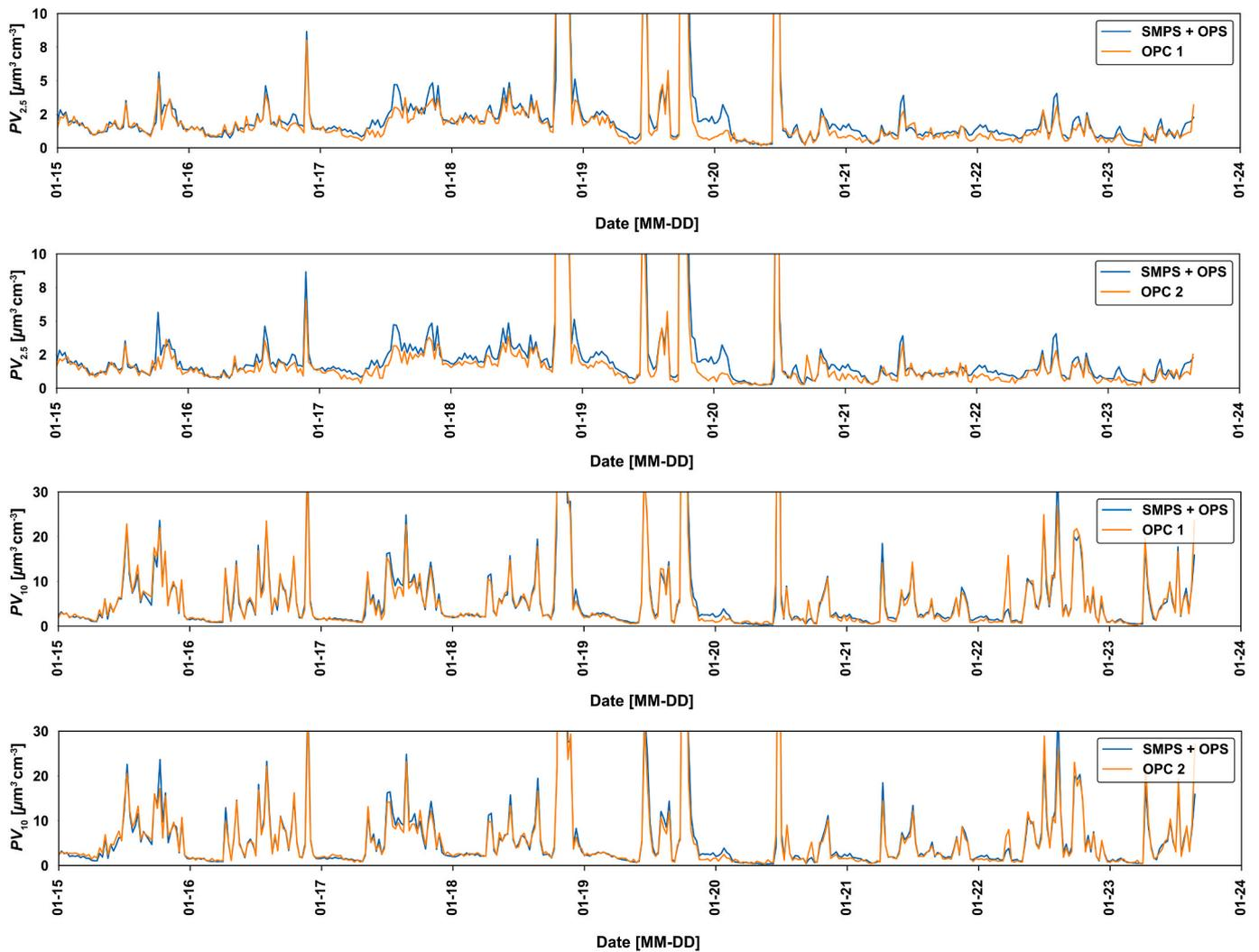
**Fig. 8.** Comparison of the corrected  $PV_{2.5}$  and  $PV_{10}$  concentration time-series reported by OPC 1 and OPC 2 with  $PV_{2.5}$  and  $PV_{10}$  concentration time-series reported by the reference instruments (OPS and SMPS) during the testing set.
