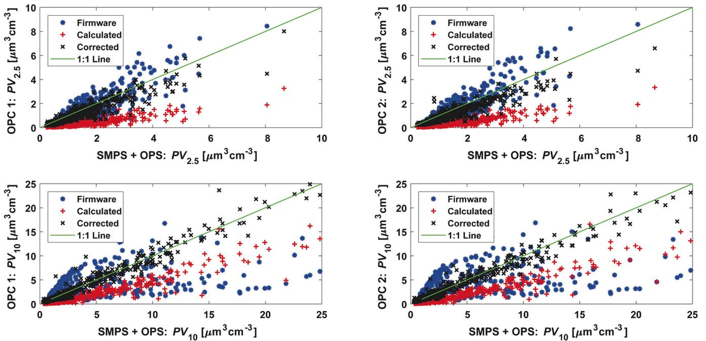
Fig. 10. Correlation plots of the calculated and firmware (uncalibrated) and corrected  $PV_{2.5}$  and  $PV_{10}$  concentrations reported by OPC 1 and OPC 2 with those reported by the reference instruments (OPS and SMPS) during the testing set.
