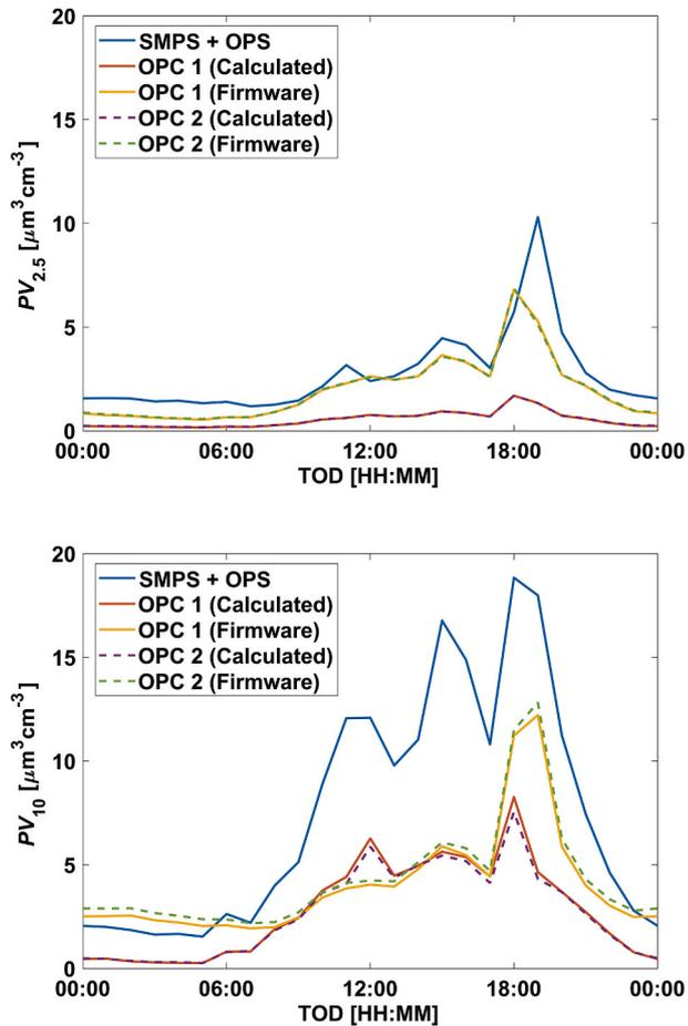
Fig. 3. Comparison of diurnal profiles in the mean  $PV_{2.5}$  and  $PV_{10}$  concentrations as reported by OPC 1 and OPC 2 (both calculated and firmware) with those reported by the reference instruments (OPS and SMPS) during occupied periods at the Purdue ReNEWW House.
