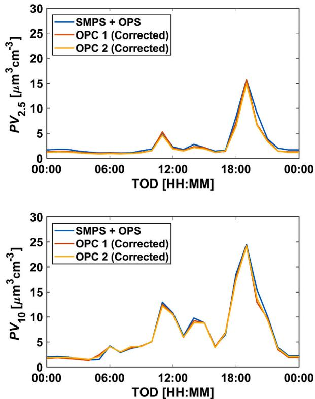
Fig. 9. Comparison of diurnal profiles in the mean corrected  $PV_{2.5}$  and  $PV_{10}$  concentrations as reported by OPC 1 and OPC 2 with those reported by the reference instruments (OPS and SMPS) during the testing set.
