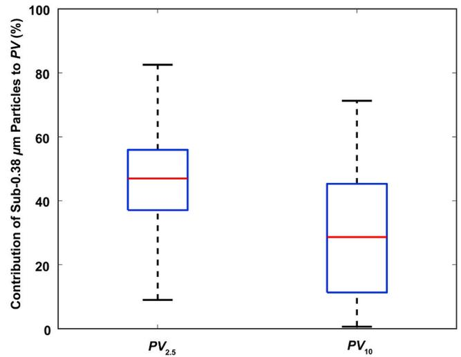
Fig. 5. The contribution of sub- $0.38 \mu\text{m}$  particles to  $PV_{2.5}$  and  $PV_{10}$  concentrations as measured by the OPS and SMPS over the entirety of the measurement campaign at the Purdue ReNEWW House.
