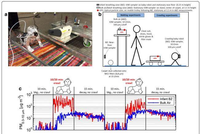
**Fig. 1** The simplified mechanical crawling infant robot with IOM sampler mounted to the robot's head and optical particle sizer (OPS) on mobile trolley (a), experimental setup of the chamber experiments (b), and example sequence of particle mass concentrations monitored with an OPS in the infant breathing zone and in the bulk air during two crawling events (c)
